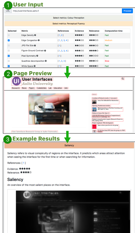
Figure 1. AIM is an online service and an open codebase for automated evaluation of GUI designs. (1) User enters URL; (2) AIM segments the image; (3) AIM presents detailed results per metric. It gives an overview of what the metric does, and an indicator of empirical evidence shown for its predictive power. A histogram offers comparison of the design to other commonly-found designs.
